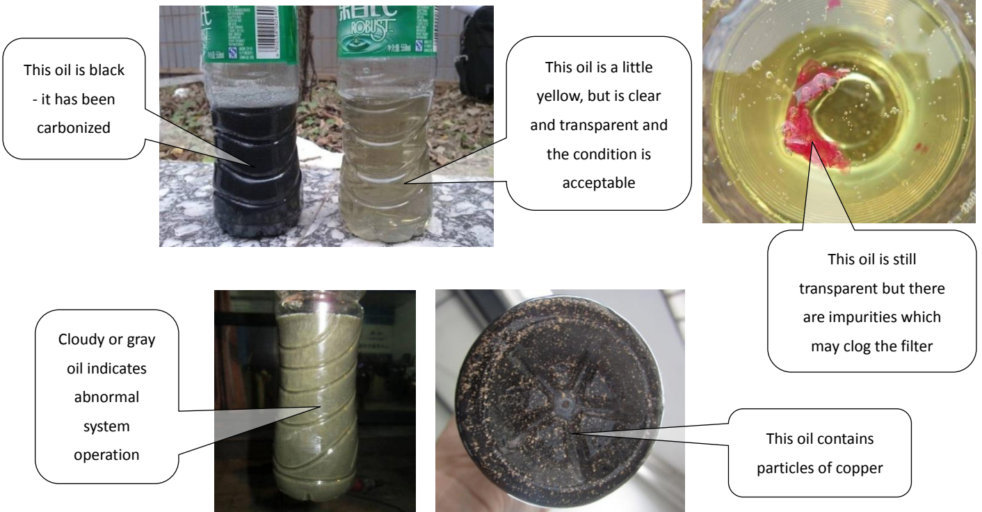
Figure 4-4.20: Inspecting compressor oil
