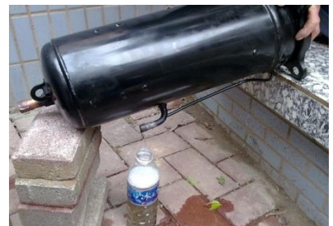
Figure 4-4.12: Draining oil from a compressor
