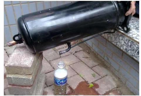
Figure 4-4.18: Draining oil from a compressor
