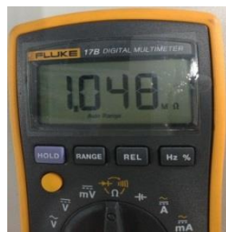
Figure 4-4.4: Measuring resistances among compressor terminals
