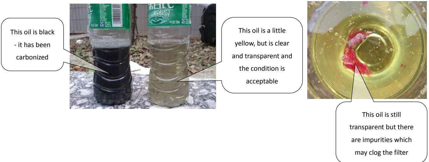
Figure 4-4.13: Inspecting compressor oil
