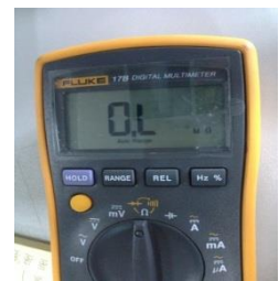
Figure 4-4.5: Measuring resistances between compressor terminals and ground
