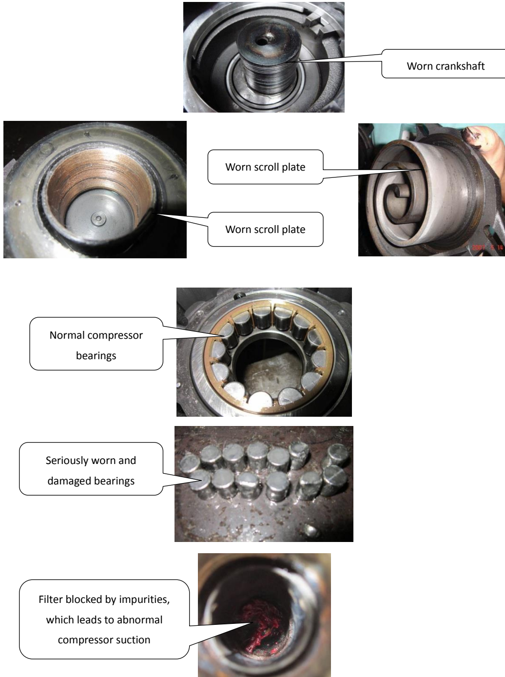
Figure 4-4.21: Effects of spoiled compressor oil
