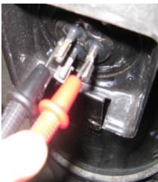
Figure 4-4.4: Measuring resistances among compressor terminals
